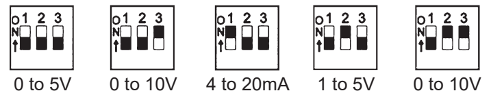
Fig. 7: DIP Switch Settings for Temperature Transmitters and Humidity Transmitters with the DIP Switches
