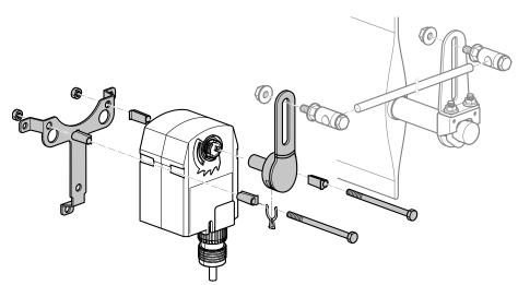
The ZG-TF2 Crank Arm Adaptor Kit can be used to replace foot mounted, crank arm style actuators. The ZG-TF2 allows for easy retrofit of Honeywell<sup>TM</sup>, Siebe<sup>TM</sup> (Barber Coleman<sup>TM</sup>), and Johnson Controls<sup>TM</sup> actuators.
