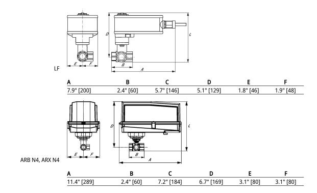
Modulating, Non-Spring Return, 24 V, for DC 2...10 V or 4...20 mA
