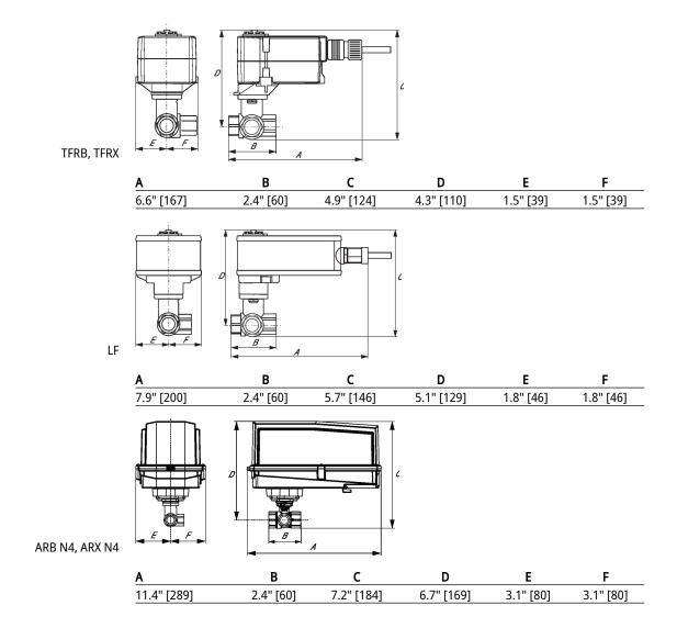
Modulating, Non-Spring Return, 24 V, for DC 2...10 V or 4...20 mA
