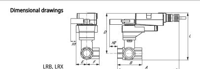
Type DN Weight [kg] [kg] B315B 15 0.30 Ε В C D H1 H2 8.5" [216] 2.4" [60] 5.2" [132] 5.0" [127] 1.3" [33] 1.3" [33] 1.2" [30] 1.1" [28]
