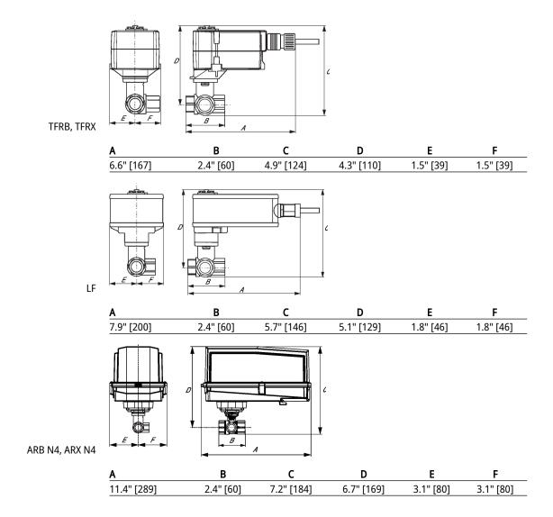
Modulating, Non-Spring Return, 24 V, for DC 2...10 V or 4...20 mA
