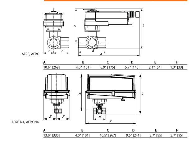
NEMA 4X, Modulating Control, Non-Spring Return, 24 V, for DC 2...10 V or 4...20 mA
