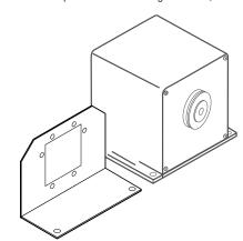
4 Match the hole pattern of the shaft face to the existing linkage and utilize the #6-32 screws and nuts with the ECON-ZIP-ACT to secure into place. **Note: At least 2 screws and nuts should be used.**
