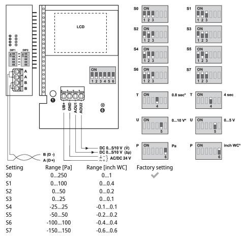
① Button ② red: Error ③ yellow: Tx ④ yellow: Rx ⑤ and ⑥ Status LED \* Factory setting P Pressure unit T Response time U Output signal
