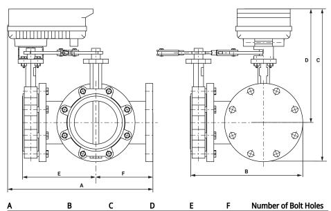
Valve with PR Actuator
