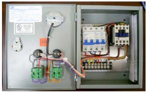
Provides Power to Operate a Single Pump Motor in Response to Two Switch Inputs, Circuit Breaker Protection and Optical & Audible High Level Alarm
